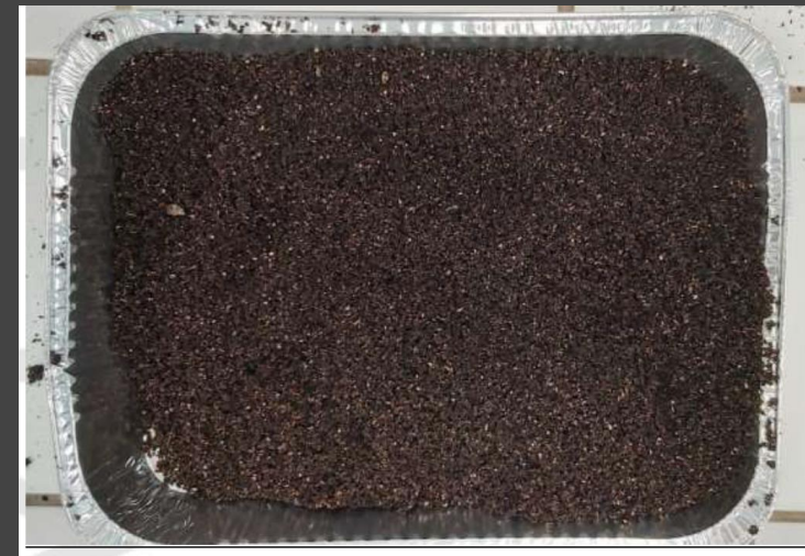
Figure 13. Sieved substrate of the final compost with test material at the end of the disintegration test
