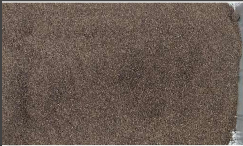
Figure 12. Sieved substrate of the sample Blank compost at the end of the disintegration test
